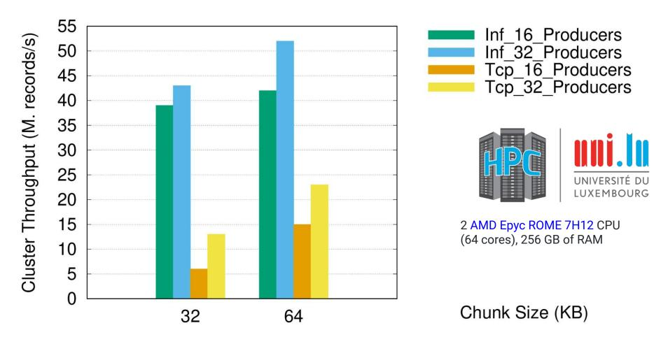
Replication factor 3, 32 streamlets with 4 groups in KerA (8 virtual logs per broker) HPC aion uni.lu, 100Gb Infiniband network, Singularity containers (RC QP) Centre for HPC 2021 National Conference
